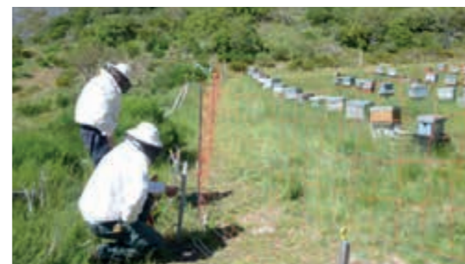
Monitoring work. Verification of the continuity of the electric discharge's intensity over time. Photo: J.M. Seijas.
